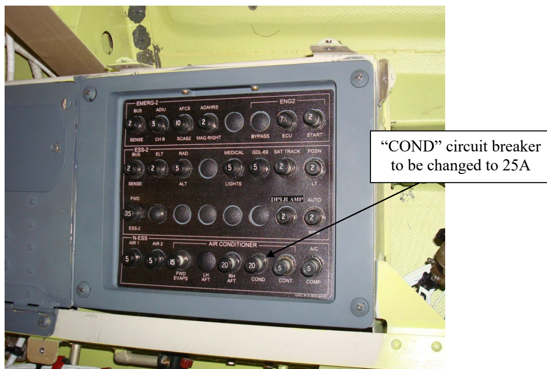
Figure 4. Circuit Breaker panel
