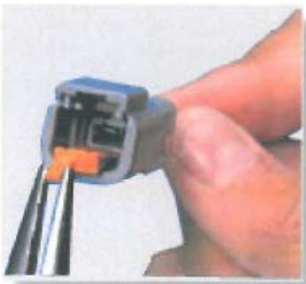
1. Remove orange wedge using needle-nose pliers to pull wedge straight out.
