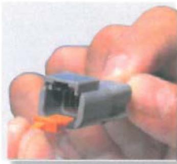
4. Once all contacts are in place, Insert orange wedge: receptades - with half holes aligning with contacts. Plugs - with contacts aligning behind full holes. The orange wedge will snap into place.
