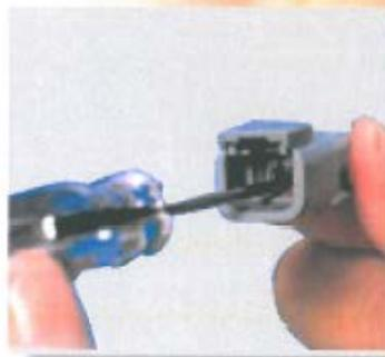
2. To remove the contacts, gently pull wire backwards, while at the same time releasing the locking finger by moving it away from the contact with a screwdriver.
