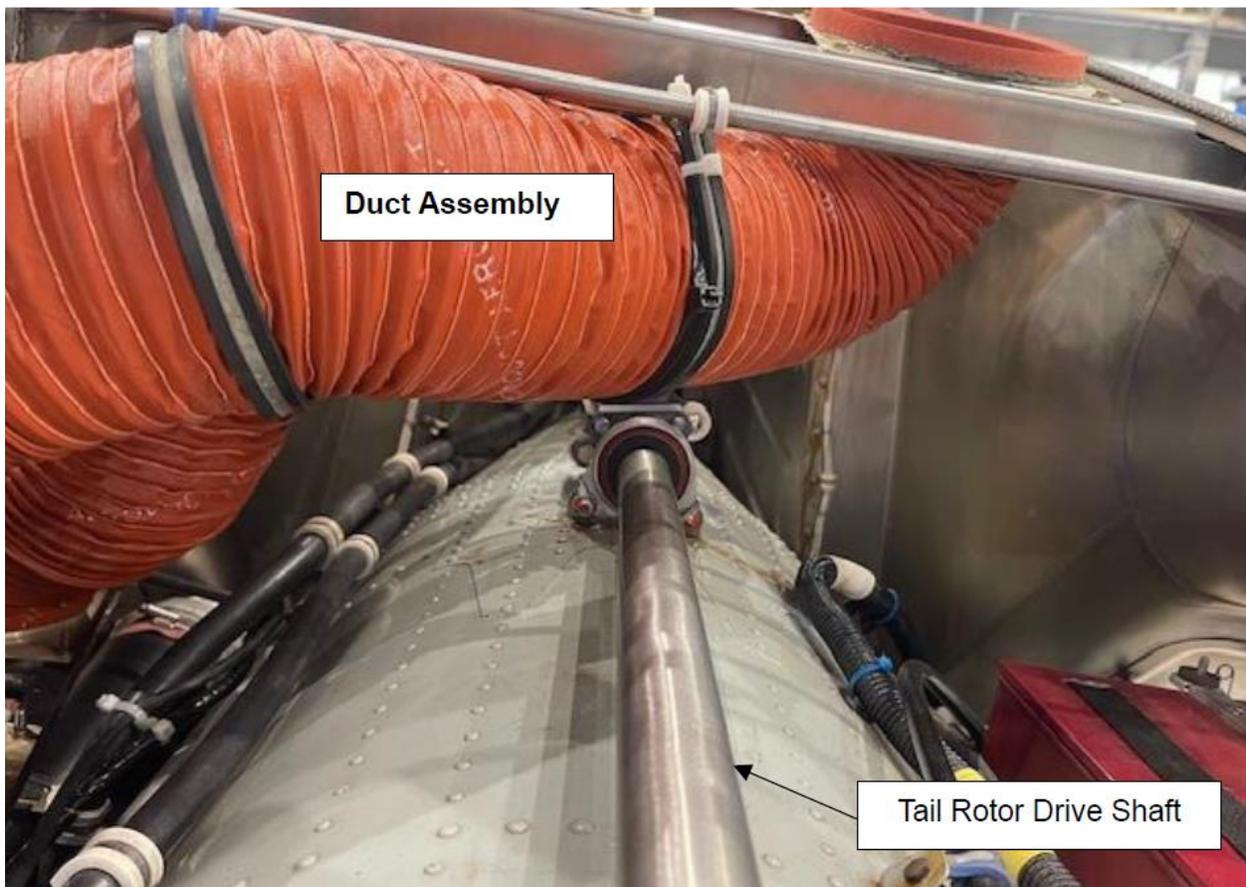
**Figure 2 – Tail Rotor Drive Shaft and Duct Installation**
