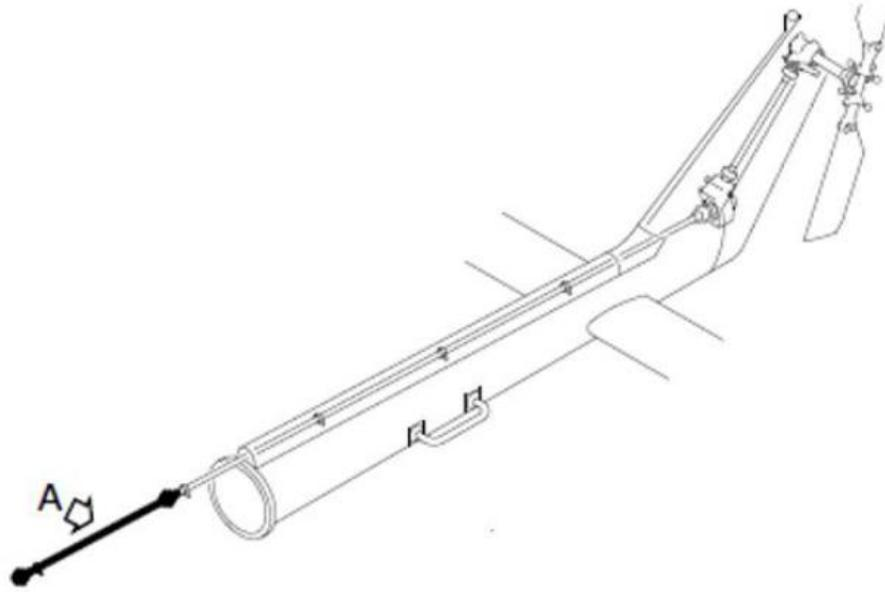
**Figure 1 – Tail Rotor Drive Shaft – Location**
