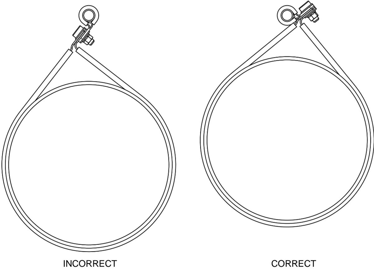
**Figure 8** – Clamp Orientation Comparison
