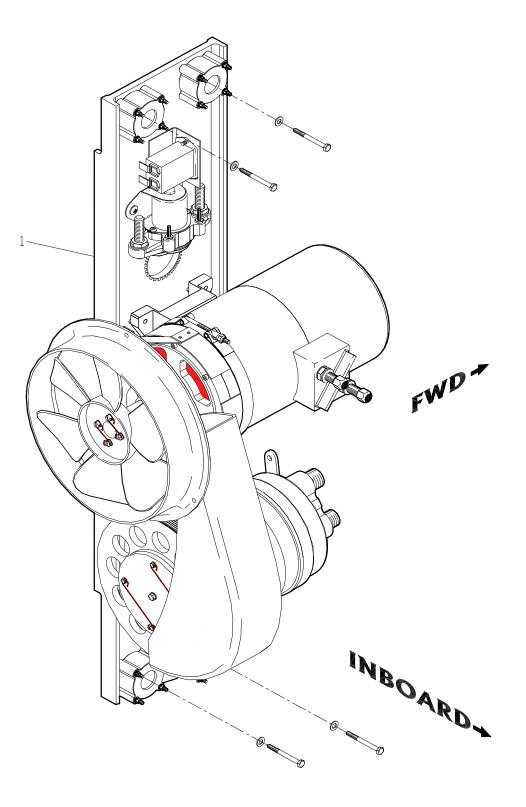
FIGURE 50 FORWARD EVAP/BLOWER INSTALLATION SHEET 1 OF 4 FIG 21-51-30 PAGE 201 June 8, 2006
