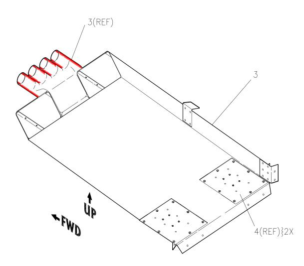
FIGURE 60 AFT EVAPORATOR INSTALLATION SHEET 8 OF 10 FIG 21-51-50 PAGE 408 June 8, 2006
