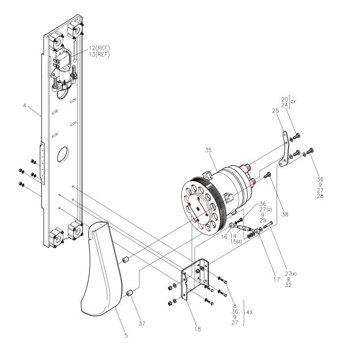
FIGURE 50 FORWARD EVAP/BLOWER INSTALLATION SHEET 2 OF 4 FIG 21-51-30 PAGE 202 June 8, 2006
