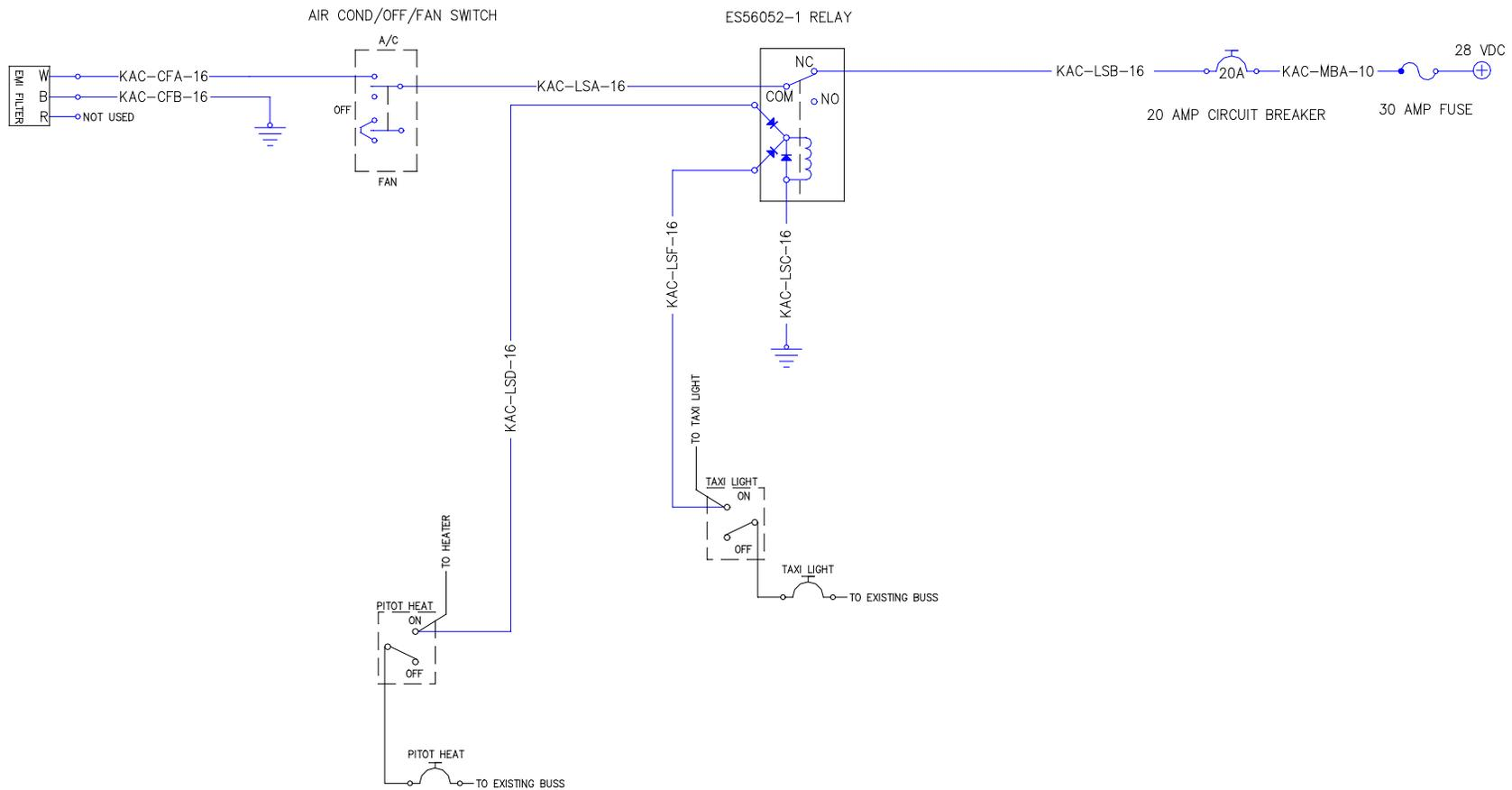
**Condenser Electrical Schematic
