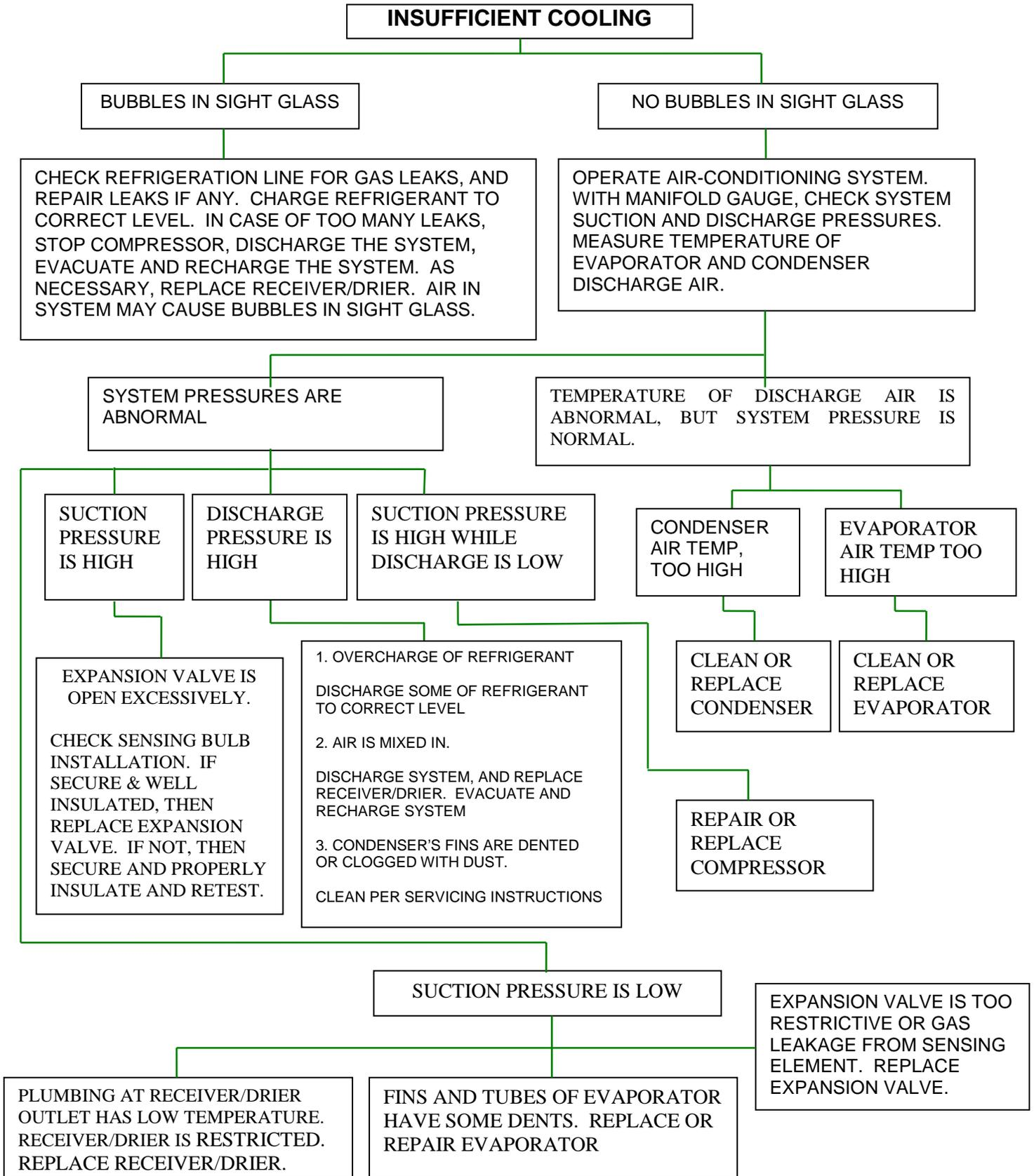
**FIGURE 2: AIR-CONDITIONING SYSTEM DIAGNOSIS CHART**
