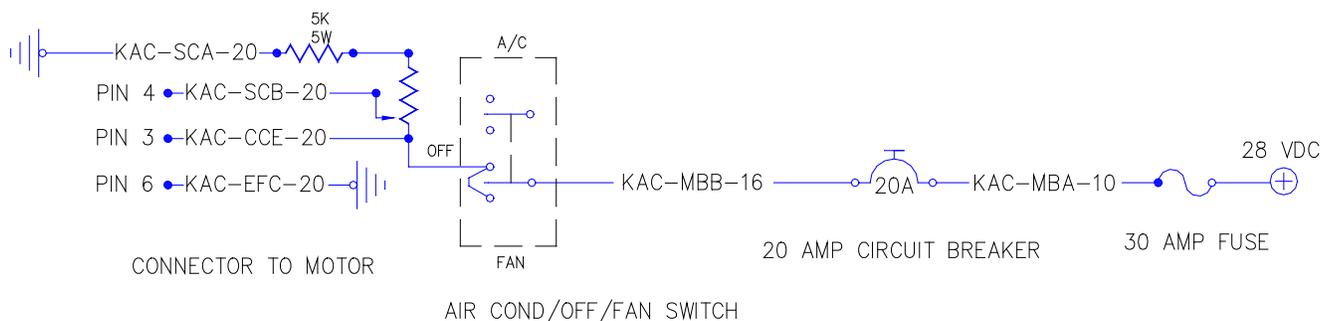
Evaporator Electrical Schematic
