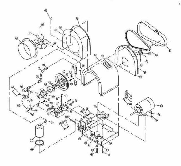
JBS5001 Compressor/Condenser Pallet Assembly Figure 1
