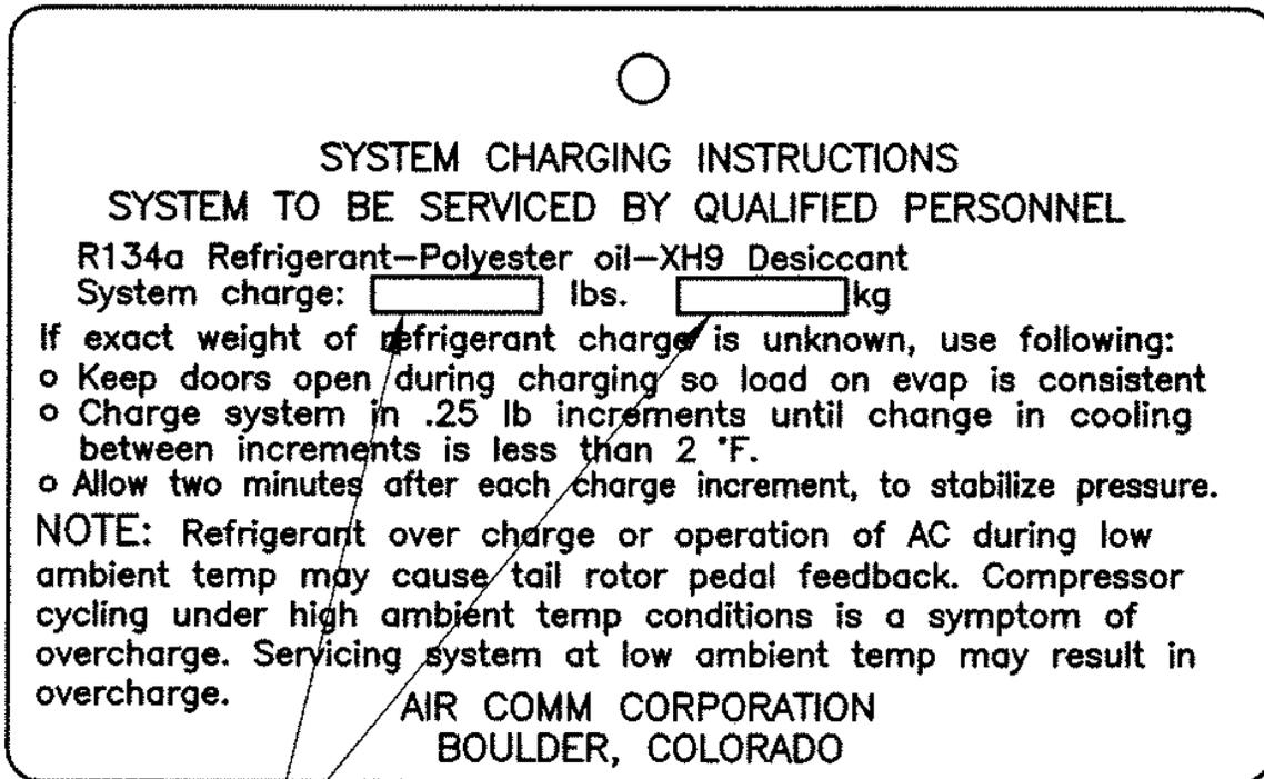
System Charge is 2.4 lb(1.1 kg) for Single Evap., 2.6 lb ( 1.2 kg) for Dual Evap.
