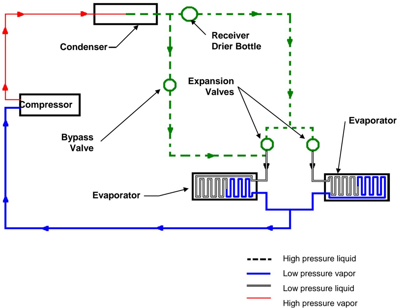
Figure 1: Refrigeration Cycle Illustration
