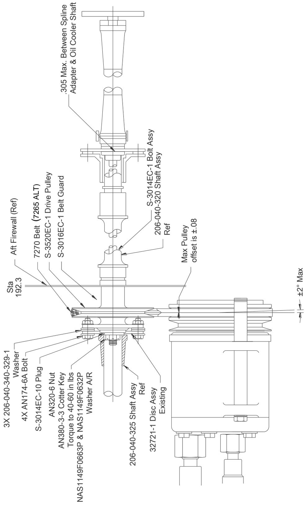
Figure 8: Compressor Belt Alignment
