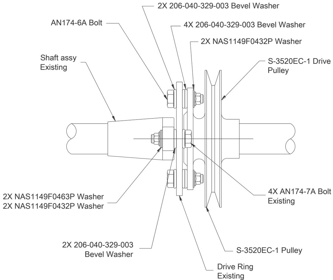
**Figure 6: Detailed View of Compressor Pulley**
