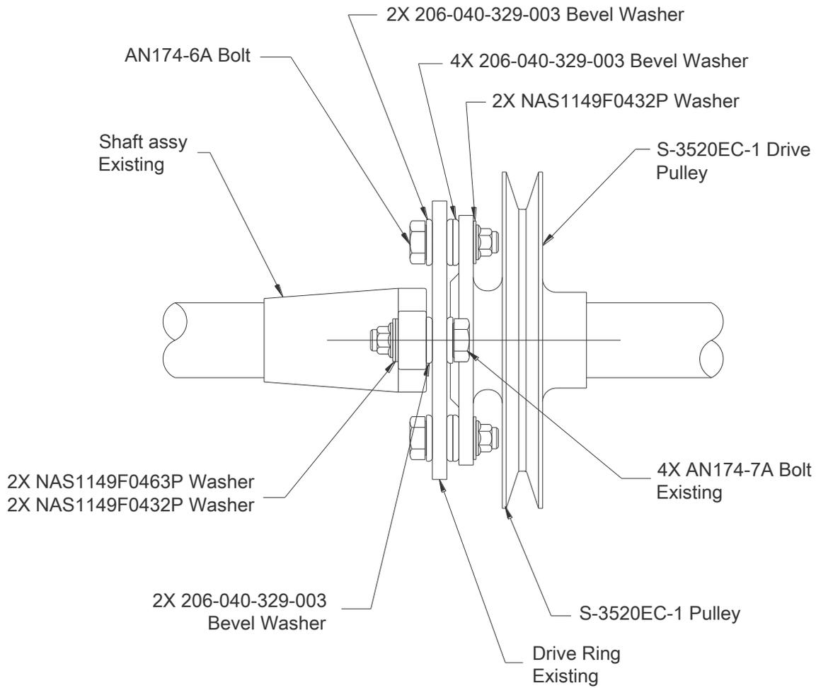
**Figure 6: Detailed View of Compressor Pulley**
