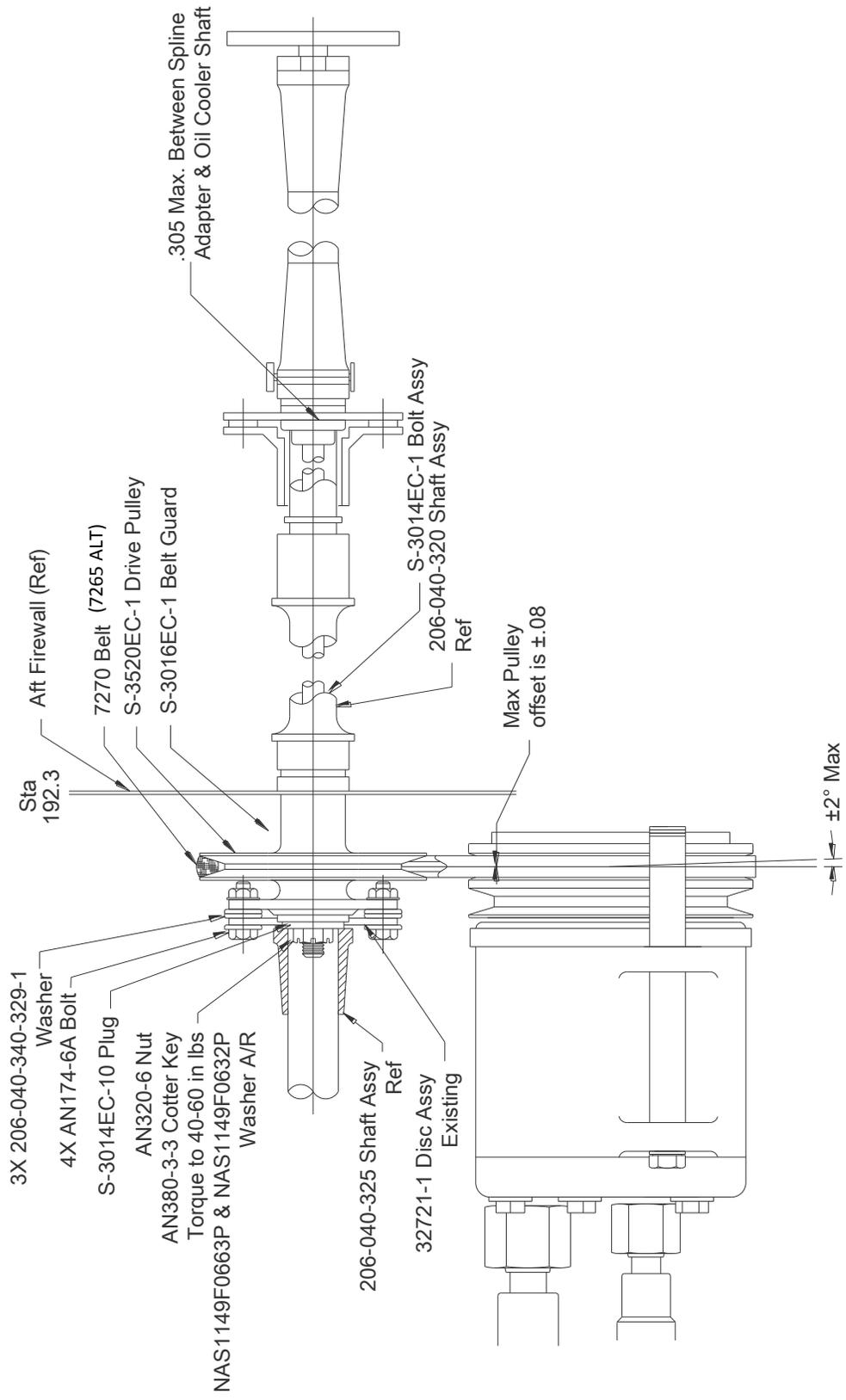
**Figure 8: Compressor Belt Alignment**
