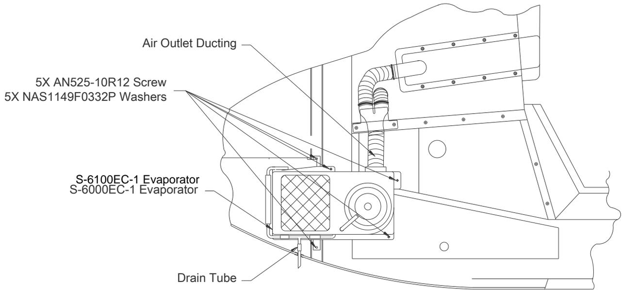
**Figure 13: Forward Evaporator - VIEW G-G**
