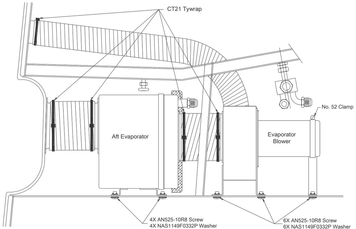
**Figure 14: Evaporator Blower - VIEW G-G**
