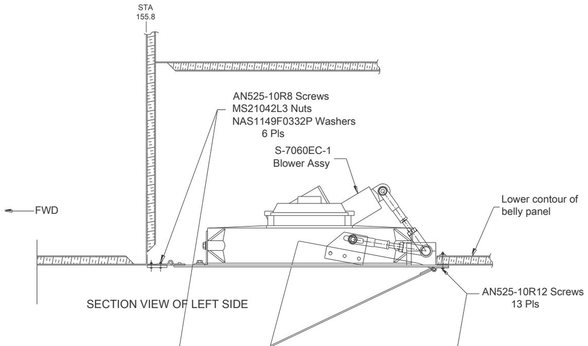
**Figure 15: Condenser Install**
