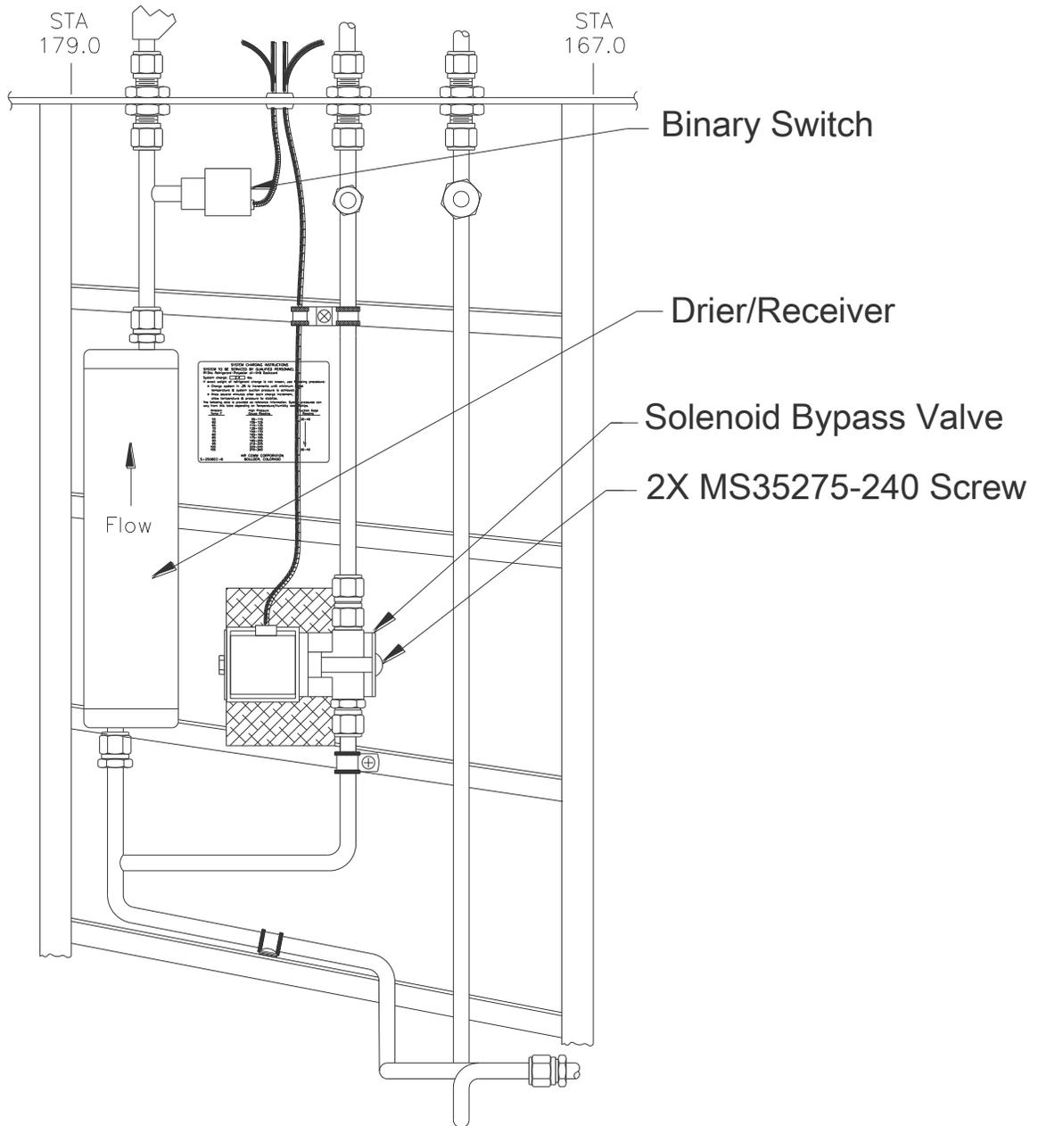
Figure 18: Binary Switch - VIEW F-F
