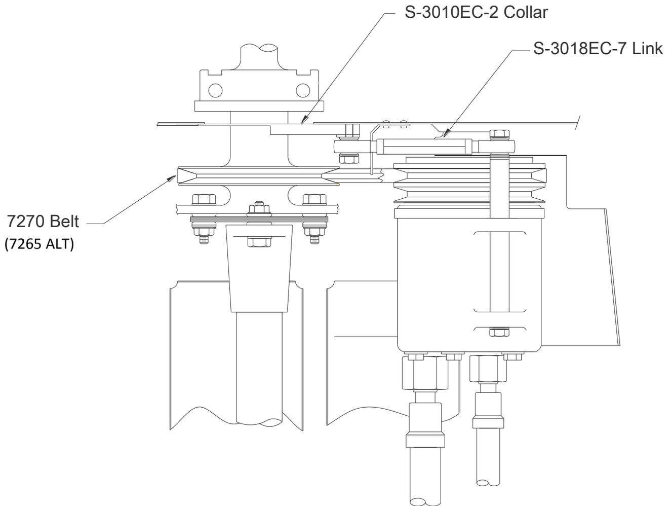
**Figure 7: View of Compressor Drive**
