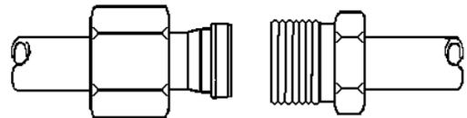
Apply a thin coating of refrigerant oil to O-Ring and Female side of fitting.
