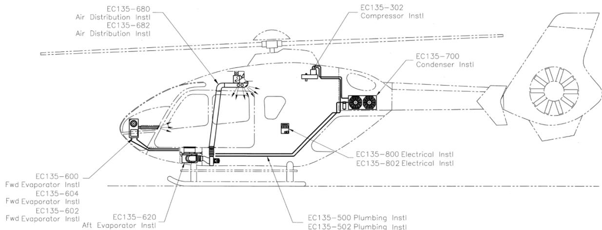
**Figure 3: Layout of Air Conditioner Dual/Single Evaporators (Side View)**
