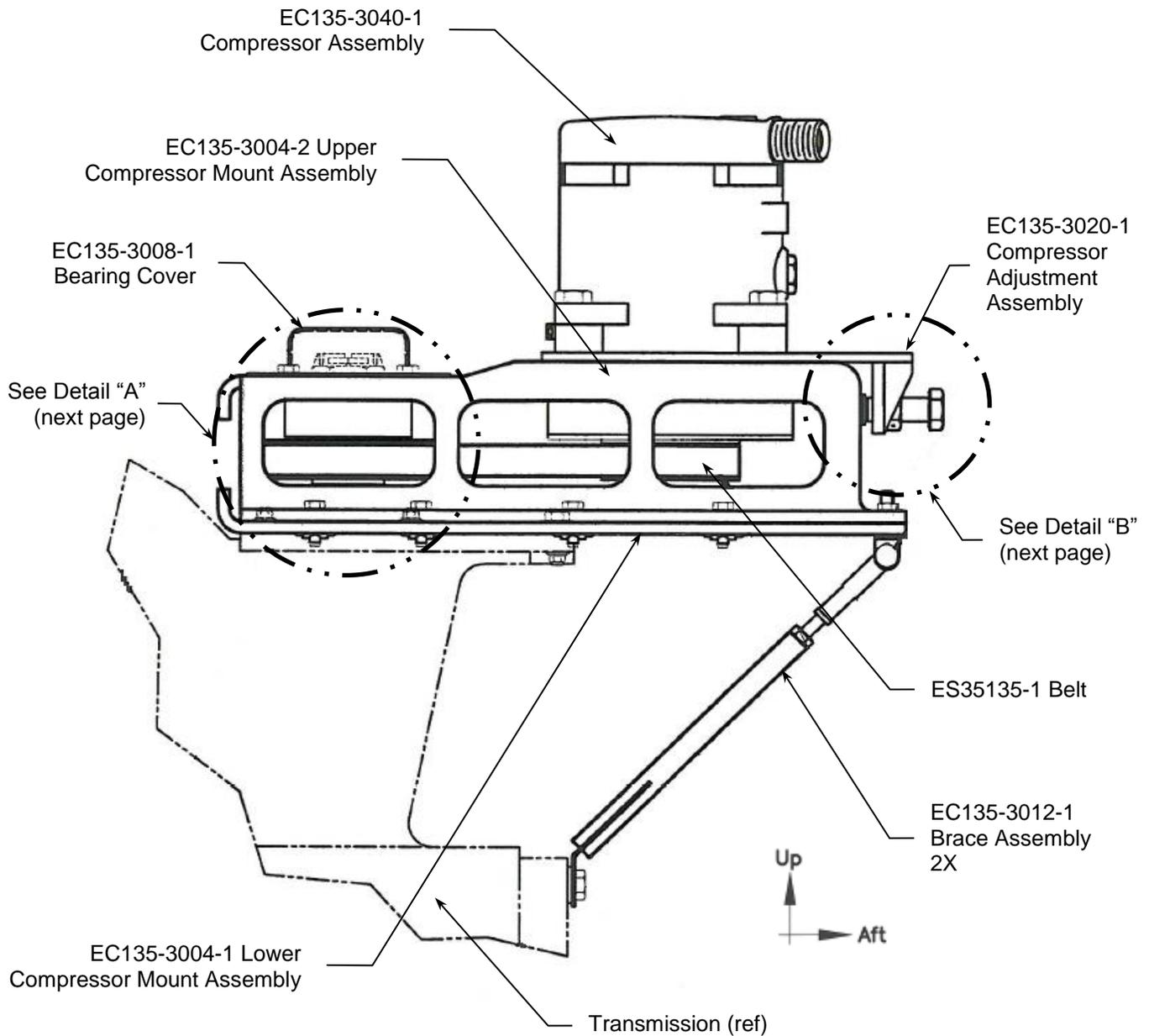
**Figure 5: Compressor Installation
