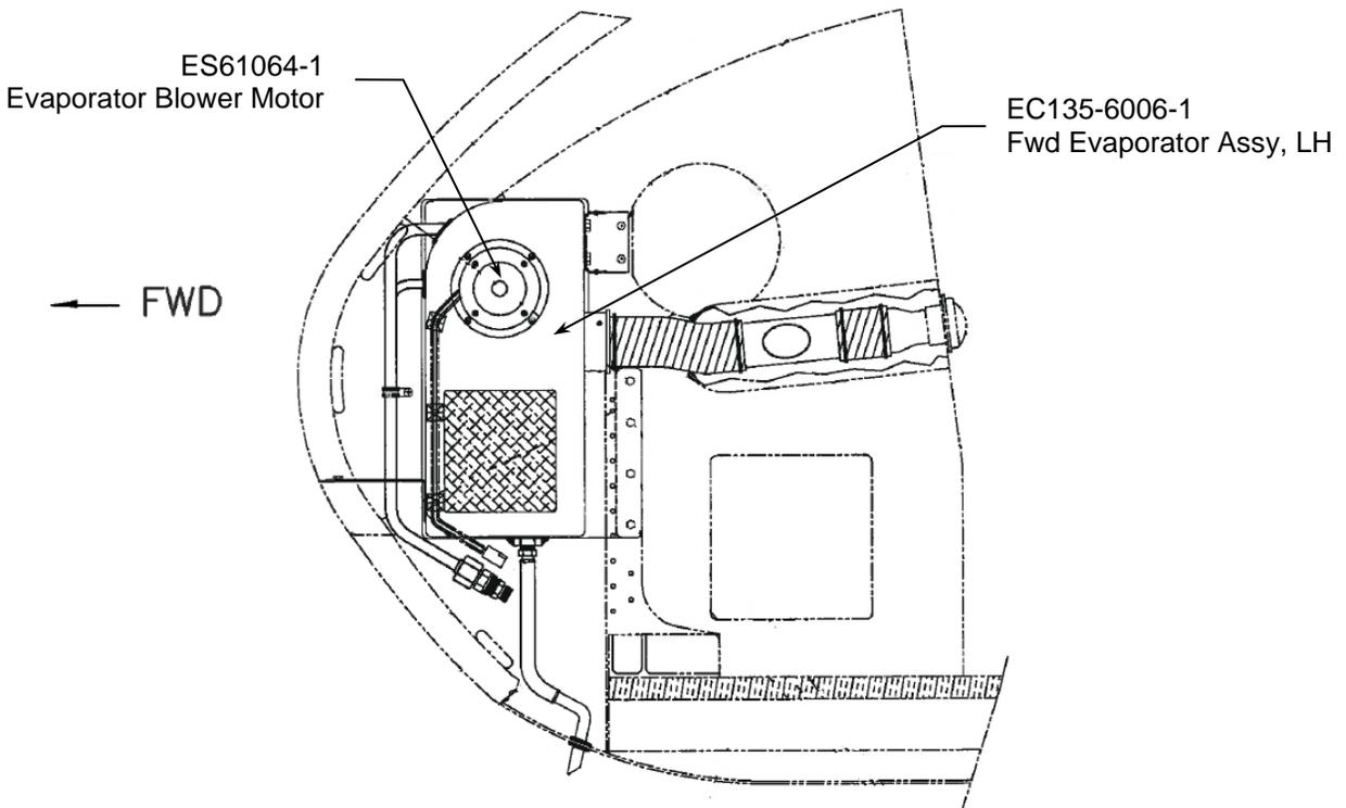
**Figure 9: Fwd Evaporator Installation, LH (View Looking Inboard)**
