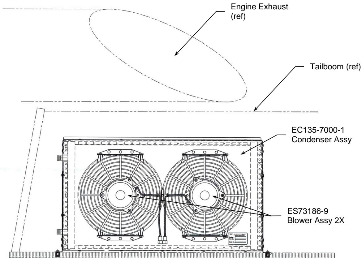
**Figure 11: Condenser Installation
