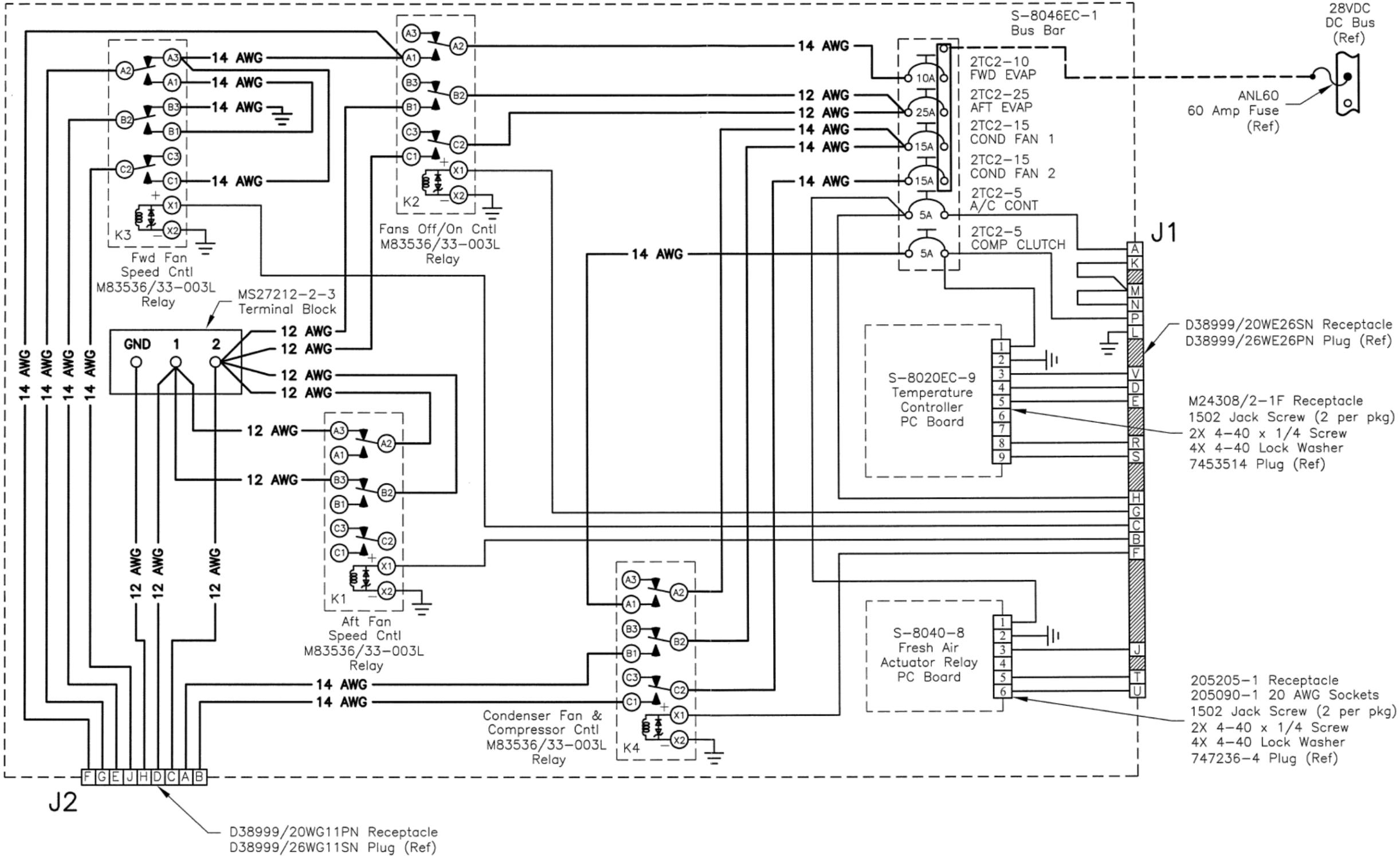
Figure 20: Relay Panel Schematic
