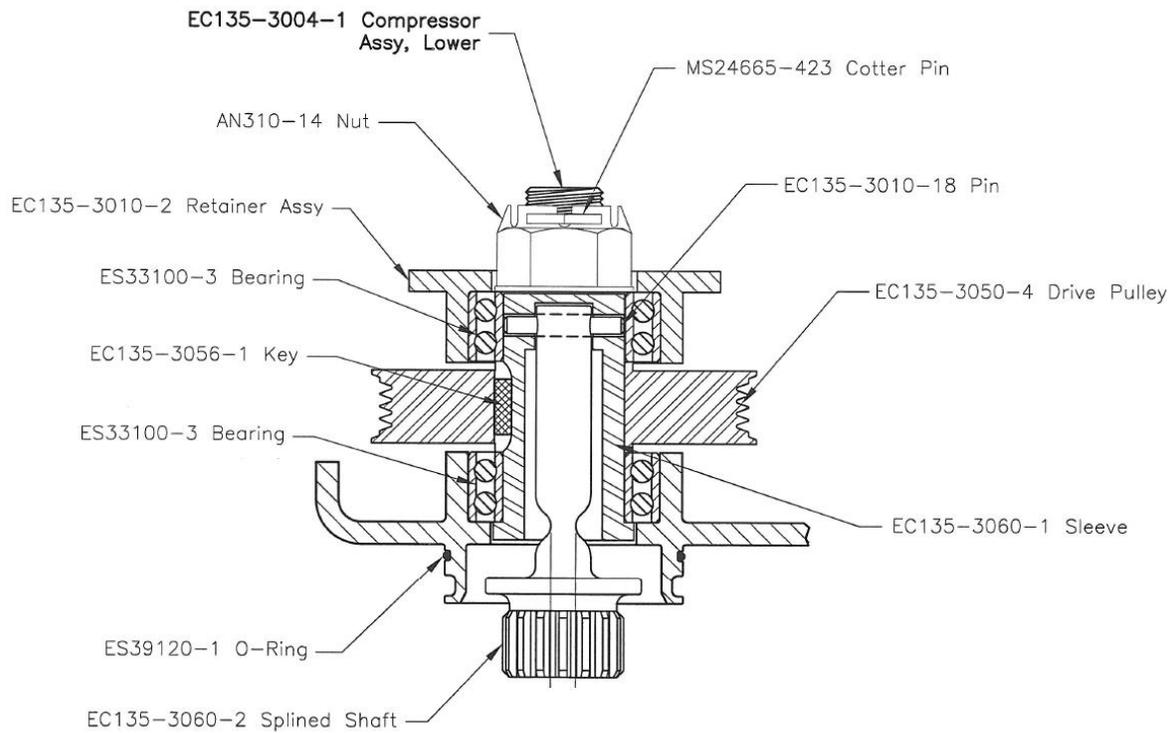
**Figure 6: Detail "A" Compressor Lower Mount Drive Pulley Assembly**
