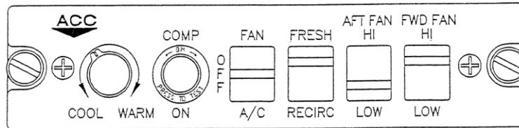
**Figure 1: Cockpit A/C Control Panel**
