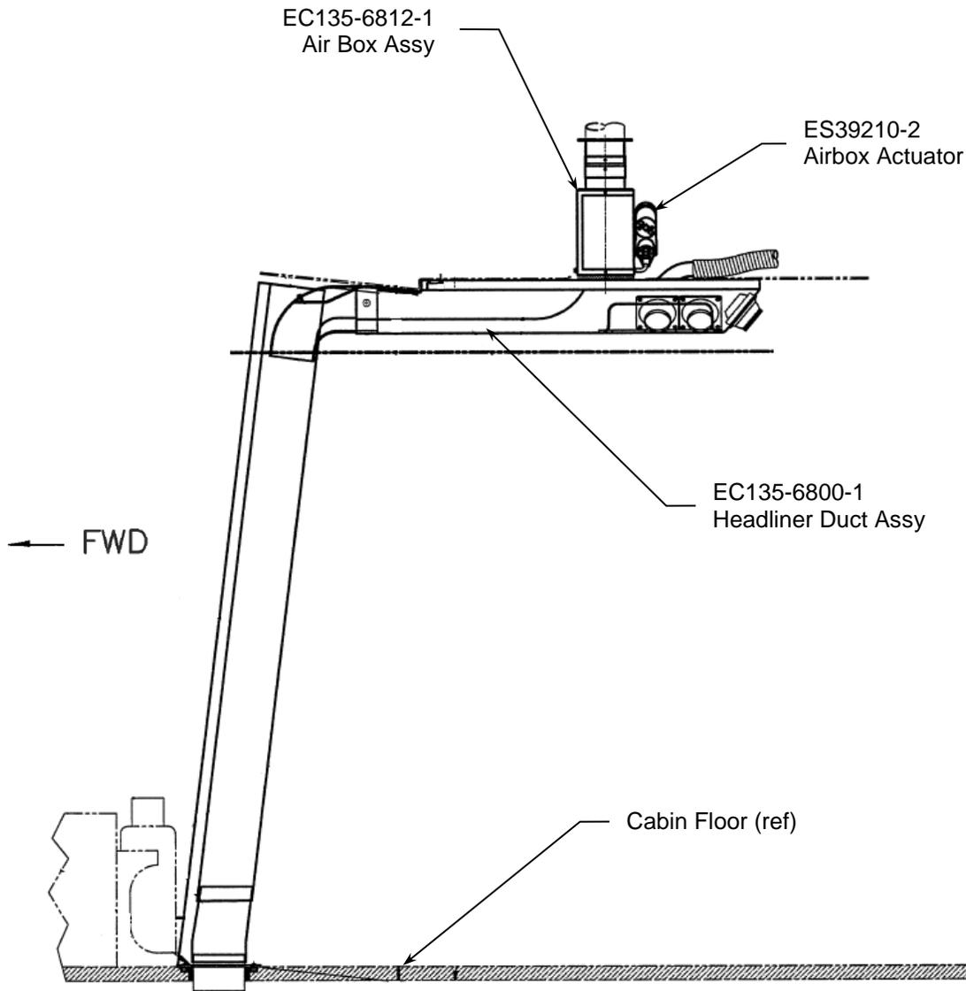
**Figure 12: Air Distribution Installation
