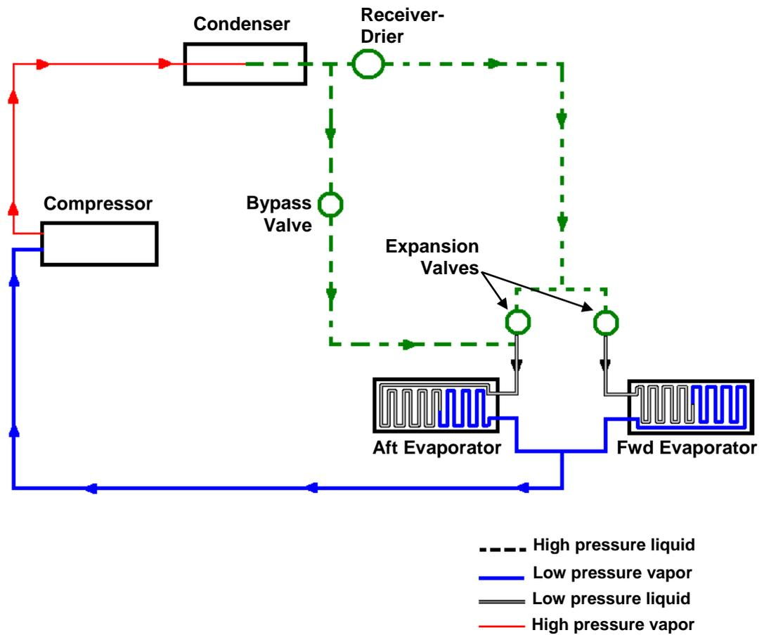
**Figure 2: Refrigeration Cycle Illustration**
