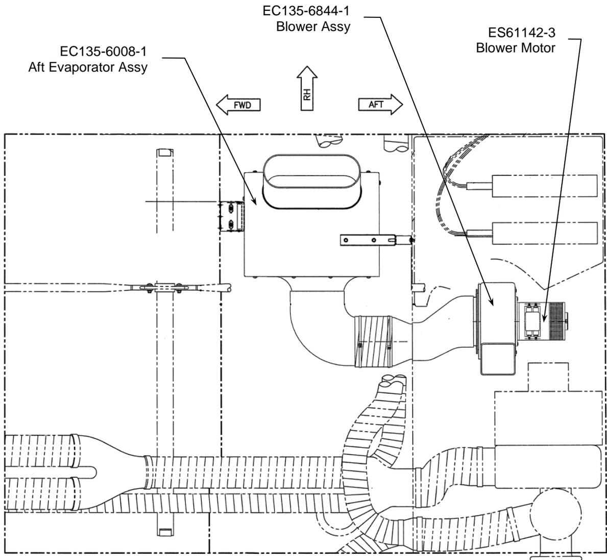
**Figure 10: Aft Evaporator Installation
